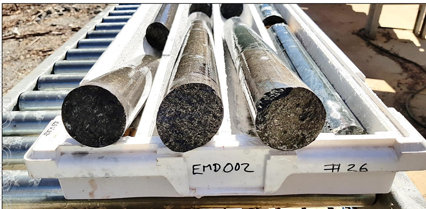
Figure 3. Matrix and semi-massive nickel sulphides intersected in EMD002 from 99.0m-101.0m.
