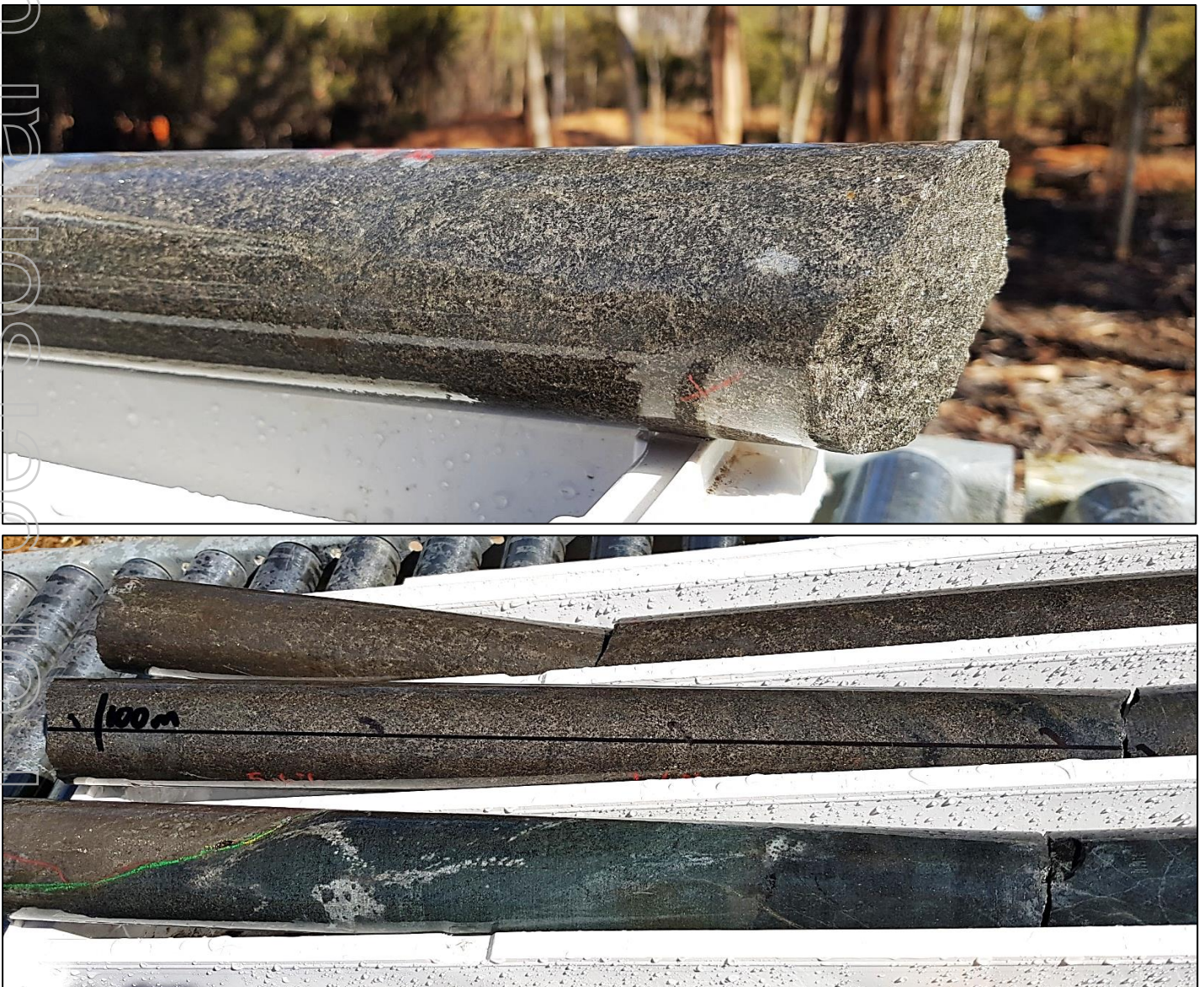
Figure 1. Close-up of matrix style nickel sulphides and basal semi-massive sulphide zones intersected in EMD002 from 99.0m –101.0m
