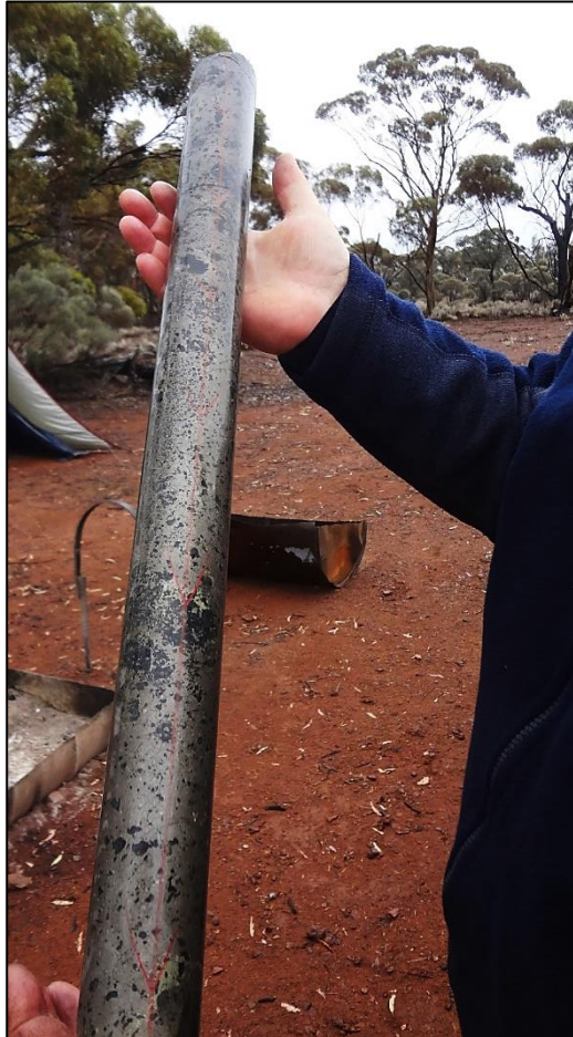
Figure 2. Ni-Cu bearing massive sulphide zone in diamond drill hole CBDD030 drilled 300m south of the T5 Ni-Cu discovery zone (436.7m-437.6m shown).
