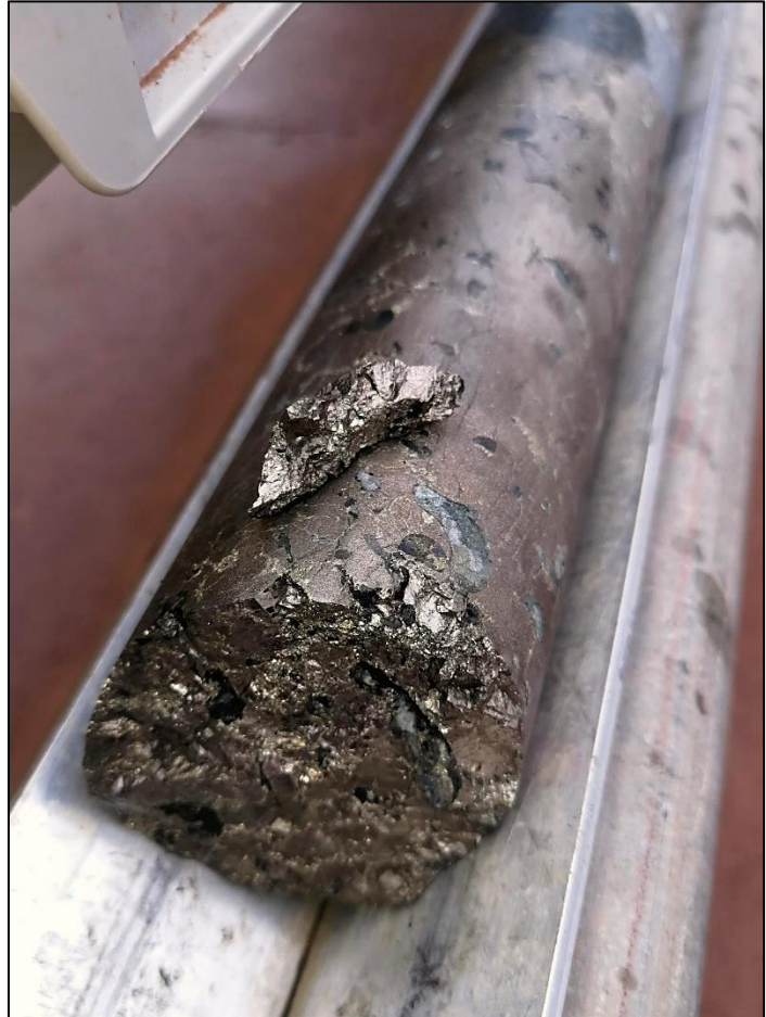
Figure 2. Ni-Cu bearing massive sulphide zone in diamond drill hole CBDD030 drilled 300m south of the T5 Ni-Cu discovery zone (436.7m-437.6m shown).
