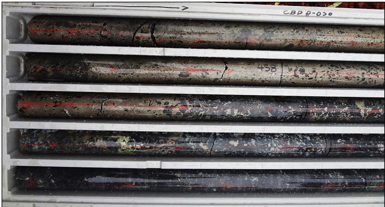
Figure 3. Unique magmatic sulphide textures showing breccia rip up clasts within the massive sulphide, interstitial sulphide/crystal intergrowth at the margin, and chalcopyrite segregation within the crystallised host gabbro. Coarse blebs of matrix sulphide are observed between the crystallising host rock (436.7m-441.1m shown).
